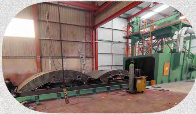
Steel Structure Shot Blasting Machine
