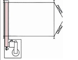
The most economical floor design available. The system contains metering shed plate, heavy duty screw belt and bucket elevator.20" air-wash separator, perforated plate rotary drum separator and oversized abrasive storage hopper with a caged man ladder and handrail. This can be expanded to an "H", "U", or full floor reclaim system and is best suited for low to medium production levels.
